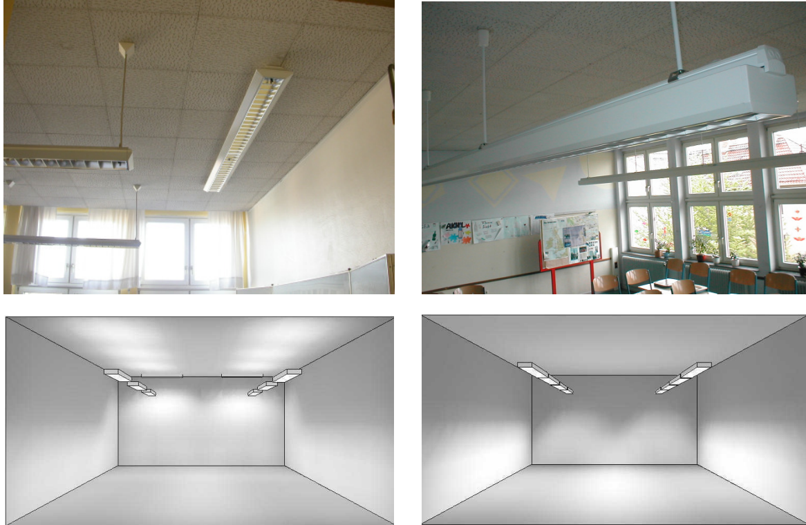
Fig. 3: lighting pilot-classroom (left): 6,1 W/m 2 , 420 lx, comparison classroom (right): 8,8 W/m 2 , 670 lx
